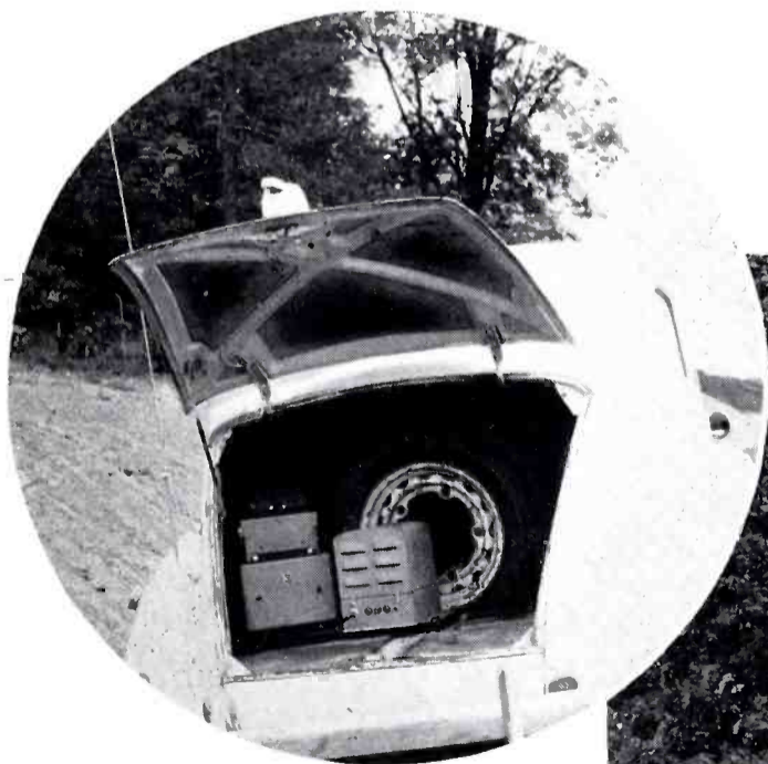
▲ Two-way radio set is installed in all motor police patrol cars. In case of an emergency the patrolman on duty can receive as well as send messages to various control points along the super highway.
